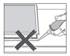
Do not use any sealant unless expressly instructed to do so. The sealing strip under the edge of the top part of the appliance provides a sufficient seal for the worktop.
